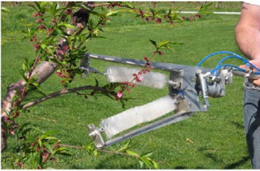
Fig. 8 Prototype end effector for automated blossom selective thinning [25]
