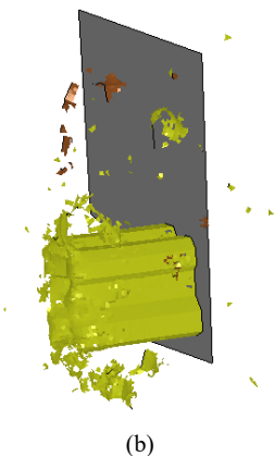
Fig. 6 Results for medium radius: (a) velocity and deceleration vs. stroke, (b) final deformation of the longitudinal crash box
