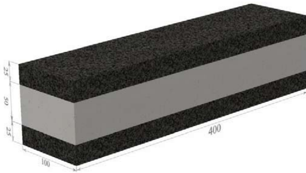
Fig. 13 Three-layer fiberconcrete (layers with fibers on the top and at the bottom)
