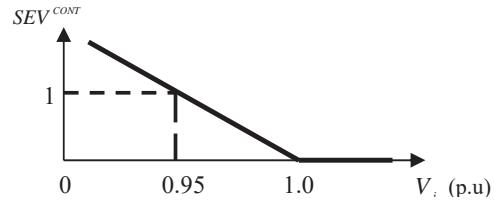
Fig. 1 Continuous severity function for low voltage
