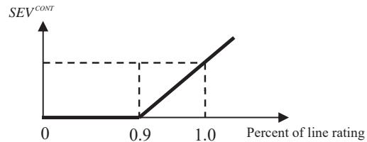
Fig. 2 Continuous severity function for line overload
