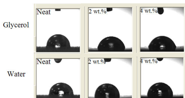
Fig. 5 Contact angle of solvents (glycerol and water) droplet of neat, 2 wt.% and 4 wt.% nanocomposites
