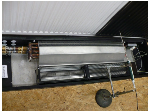
Fig. 5 Exchanger in laboratory
