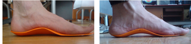
Fig. 9. Study of real compatibility between the plantar surfaces and the corrective insoles manufactured by rapid prototyping (flat foot-left, hollow foot-right)
