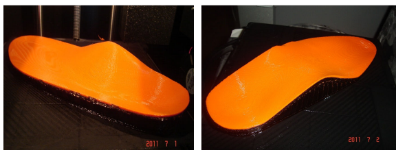
Fig. 8 Manufacturing corrective insoles using rapid prototyping method (flat foot-left, hollow foot-right)
