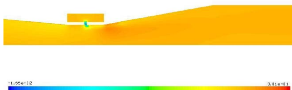
Fig. 8 Contour of velocity in perpendicular to flow direction in 12-holes mixer (m/s)
