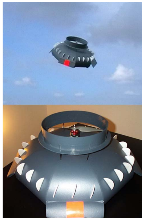
Fig. 1 A typical Coanda Saucer UAV developed and tested by Jean-Louis Naudin. The diameter of the saucer is approximately 60 cm [11]
