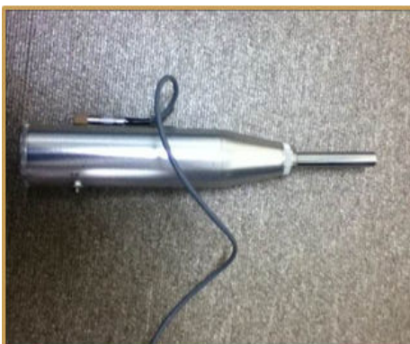
Fig. 1 Schmidt hammer before waterproof
