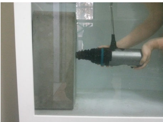
Fig. 6 Rebound Hardness Test in under water condition
