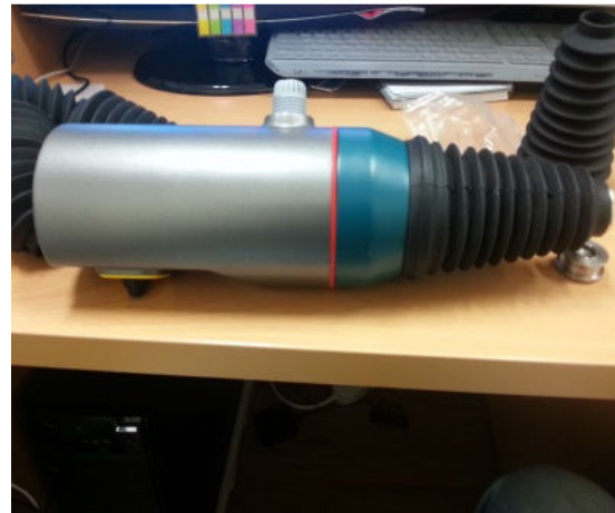
Fig. 2 Schmidt hammer after waterproof
