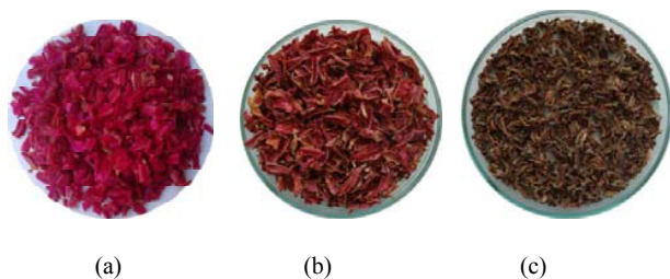
Fig. 3 Example of o dragon fruit peel; a) fresh peel b) drying at 110 °C c) sun drying
