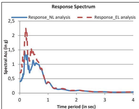
Fig. 22 Response spectrum for BH-2 CH-57.769 km
