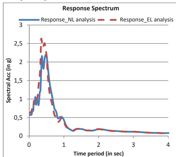
Fig. 19 Response spectrum for BH-1 CH-53.769 km
