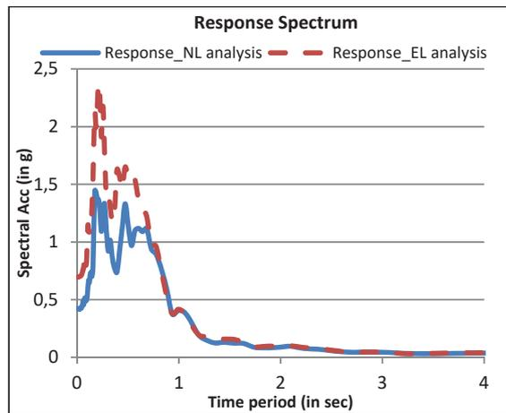
Fig. 21 Response spectrum for BH-1 CH-57.769 km
