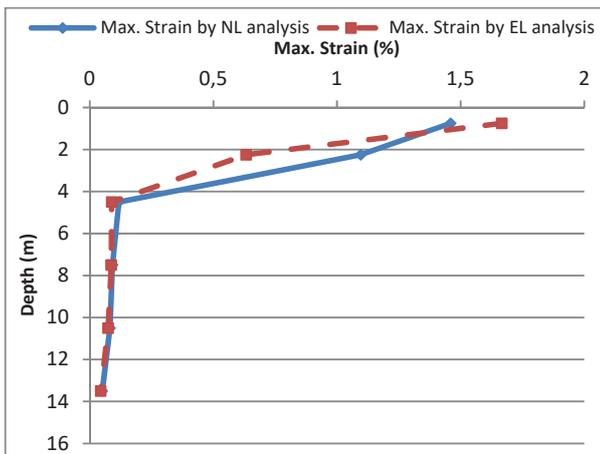
Fig. 16 Maximum Strain with Depth of soil column BH-1 CH-57.769
