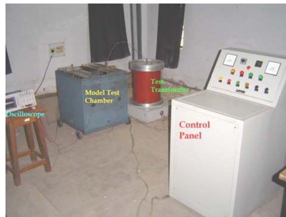
Fig. 2 Photograph of experimental setup viewing voltage source, model experiment chamber, sensors and recording device (digital storage oscilloscope)
