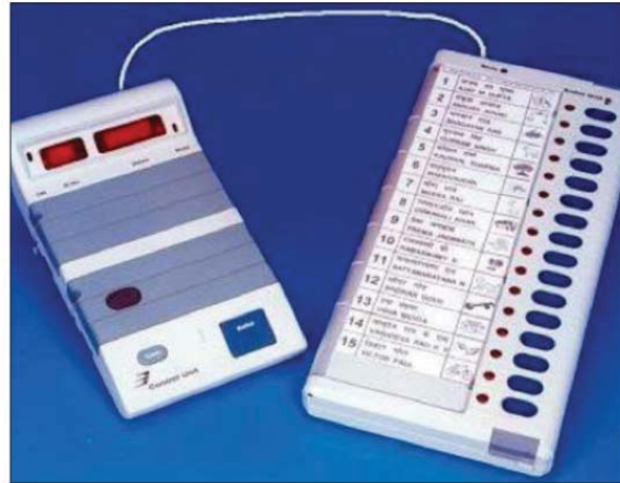
Fig. 4 Electronic Voting Machine-Control Unit and Ballot Unit [19]
