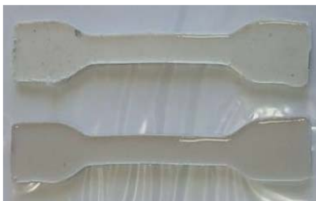
Fig. 6 Moulded Ag doped CNFs/RTV664 composite
