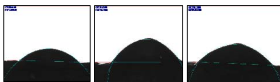
Fig. 8 Sessile drop images for (a) 5% lignin, (b) 20% lignin onto urea surface
