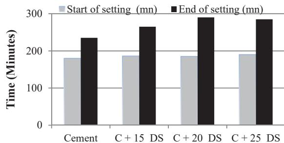
Fig. 4 Initial and End time of setting
