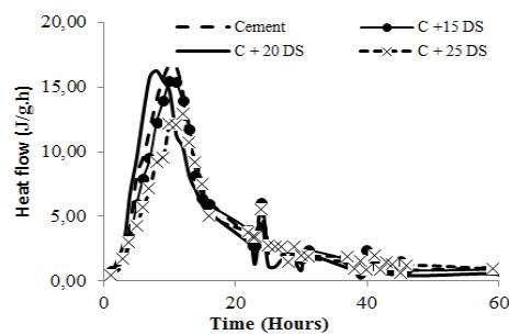
Fig. 8 Heat flow of different mortars
