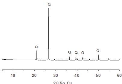
Fig. 1 X-ray diffraction pattern of ground quartz (DS)
