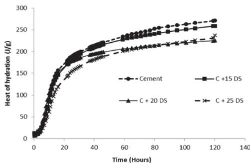
Fig. 7 Heat of hydration of different mortars at the 5 days of hydration
