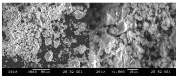
Fig. 2 SEM views of ground quartz (DS)
