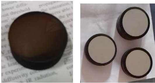
Fig. 2 Polished graphite target (a) and steel polished substrate (b)
