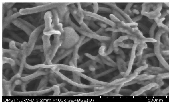
Fig. 8 FESEM images of MWCNTs-calix[8]arene with  $\text{Cd}^{2+}$
