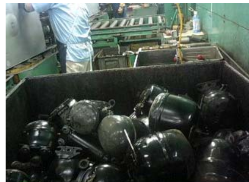
Fig. 6 Compressors Divided from Waste Home Appliances
