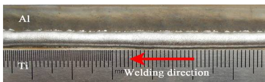
Fig. 2 Appearance of Al/Ti lap joint made by BC-MIG
