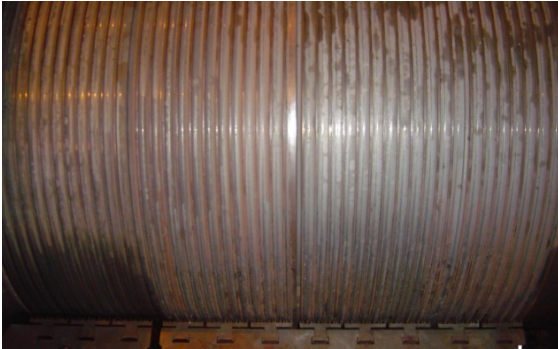
Fig. 1 Effects of rubbing on rotor surface
