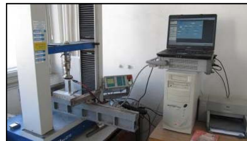
Fig. 2 Evaluation of electrical properties under loading
