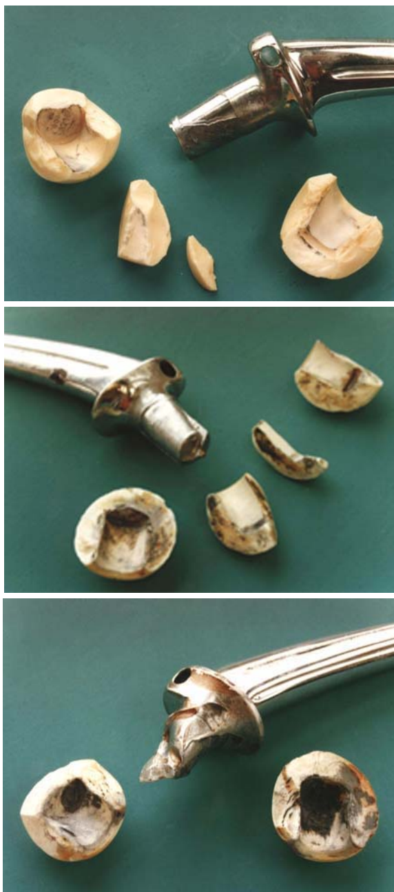
Fig. 1 In vivo destructed ceramic heads
