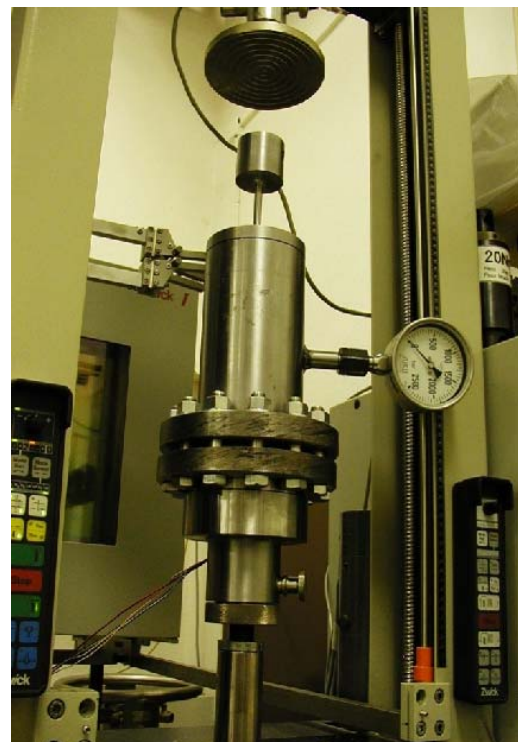
Fig. 4 Experimental jig fixed in the ZWICK testing machine
