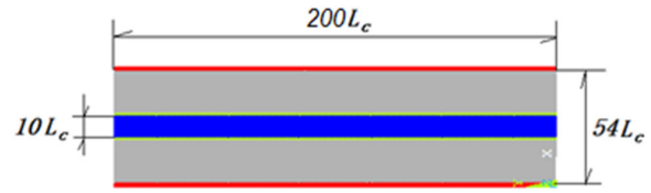
Fig. 5 Dimension of a plate with a centered fiber. Gray represents matrix, blue for fiber, green the interface and red lateral boundary
