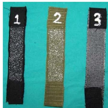
Fig. 1 Example Specimens prepared for uniaxial tensile testing
