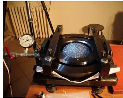
Fig. 3 Pneumatic Bulge Test Assembly
