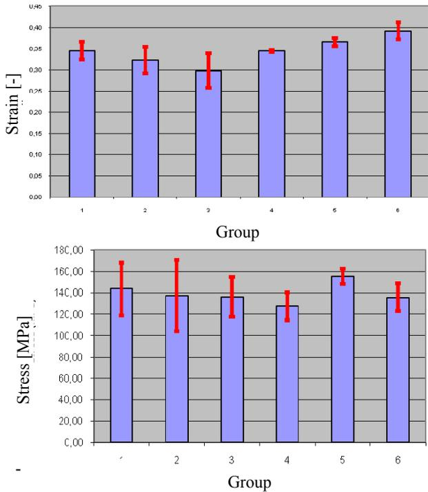
Fig. 4 Stress/Strain Results of Uniaxial Tests at Failure
