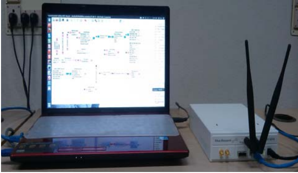
Fig. 3 Software Defined Radio development test bed
