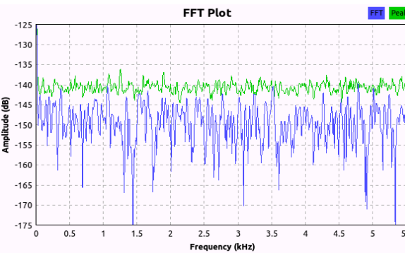
Fig. 10 Test statistic and PSD for 103.45 MHz FM signal
