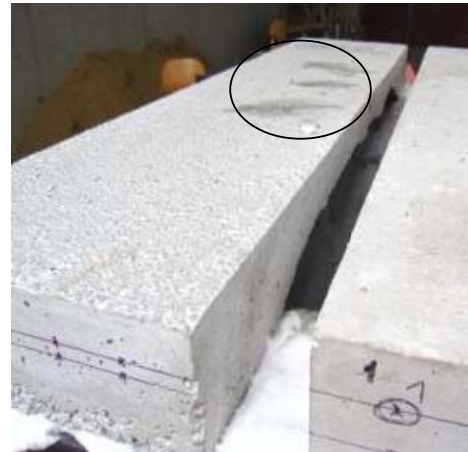
Fig. 3 Surface of the slab after thermal treatment – evaporation of water
