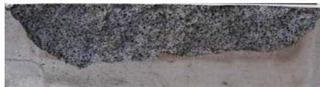
Fig. 4 State after testing – spalled concrete
