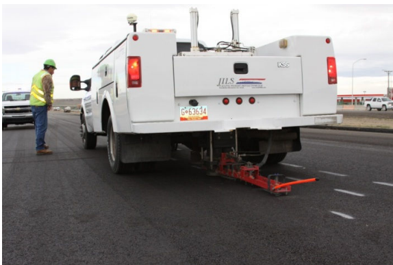
Fig. 7 Conducting FWD test
