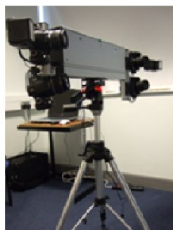
Fig. 2 The Di3D stereophotogrammetry system connected to the laptop with Di3dCapture installed
