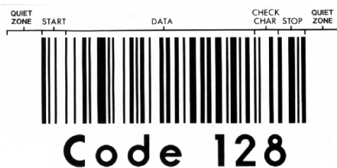
Fig. 2 Standard Code 128 Barcode
