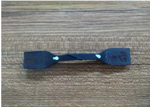
Fig. 2 Specimen is tested at 0.5 mm/s
