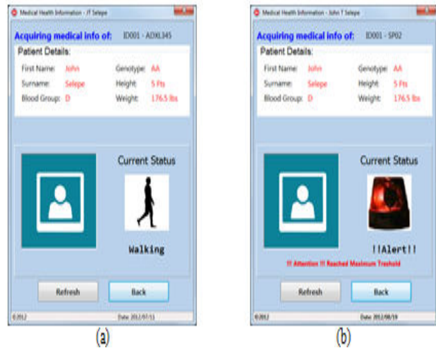
Fig. 8 Screenshots of the CIN's GUI showing (a) patient walking (ID – 3) on accelerometer monitoring and (b) an alert message in case of an emergency on pulse oximeter monitoring
