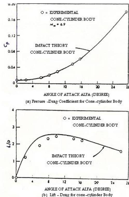
Fig. 1 CD and L/D for cone-cylinder Based on Newtonian Theory, Mach No. 6.9
