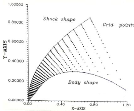
Fig. 5 Grid Point Distribution, Mach No. 5.8
