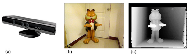
Fig. 3 Kinect motion sensing input device and the obtained data types. (a) Kinect motion sensing input device; (b) colorful images; and, (c) depth images
