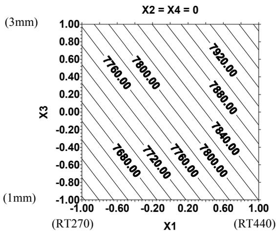
Fig. 8 Effect of material and the crack length on the maximum loading
