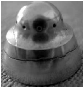
Fig. 3 A cracked tip of a nozzle body in the fuel injector of a diesel engine [26]
