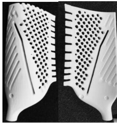
Fig. 7 Ceramic core for the blade
