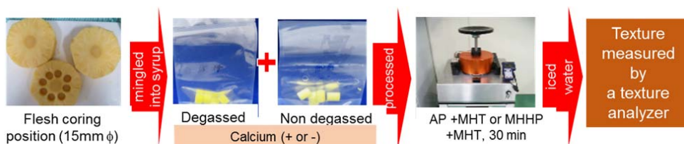
Fig. 4 Processing method of pineapple flesh
