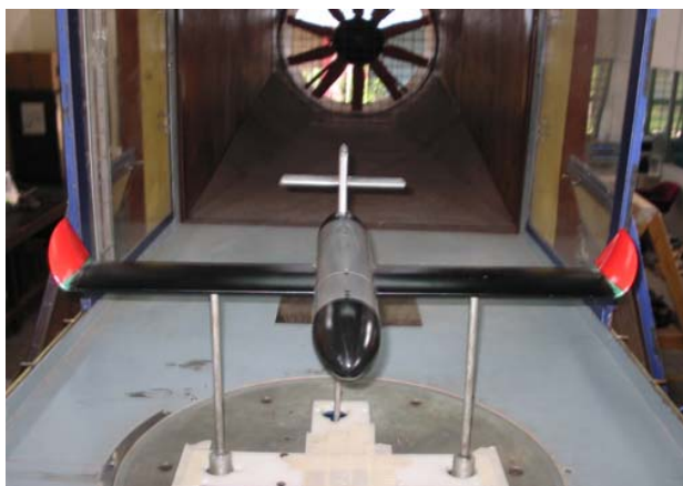
Fig.2. Aircraft Model with Elliptical shaped Winglet in test
