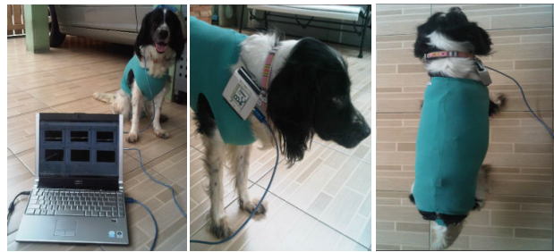
Fig. 7 Real dog with two 3-axis accelerometers at the back and tail
