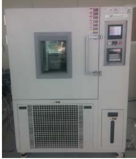
Fig. 3 Environmental (temperature) chamber used for the test
