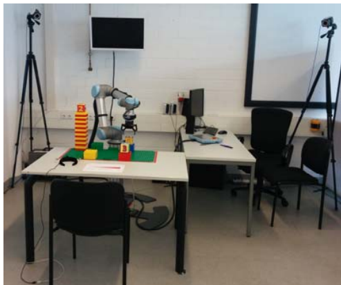
Fig. 2 Experimental setup, UR5 robot with gripper, screen, hairband with IMU, and motion capture cameras
