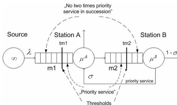
Fig.1. Illustration of the three-station network model with blocking, priority feedback service and thresholds.
