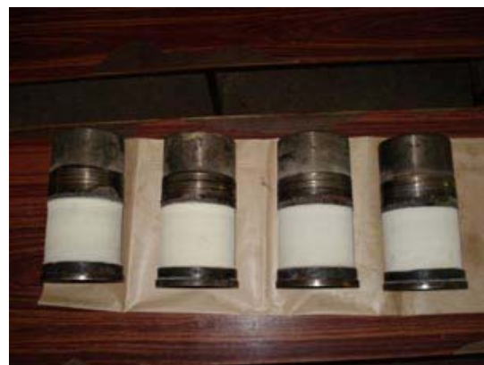
Fig. 2 Photographic View of Cylinder Liner (After Ceramic Coating)
