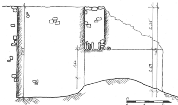
Fig. 8 Section of Lime Kiln 2
