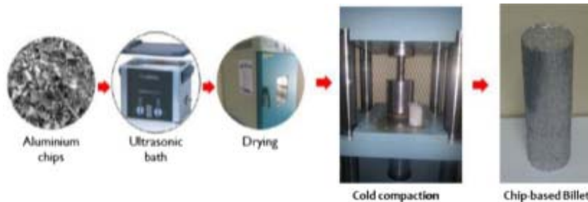
Fig. 2 Preprocessing of chips before consolidation
