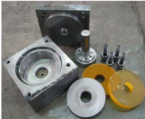
Fig. 2 Photograph of the new die set parts
