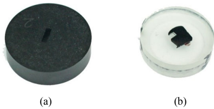
Fig. 9 Thermal effect evaluations using (a) hot mounting technique (b) cold mounting technique
