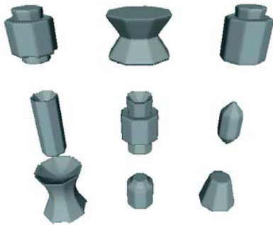
Fig. 8 The surfaces m(x, z) \otimes h(x, y) = 1 created using the curves in Figs. 5(A)-(I) as m(x, z) = 1 and the curve in Fig. 6 as h(x, y) = 1
